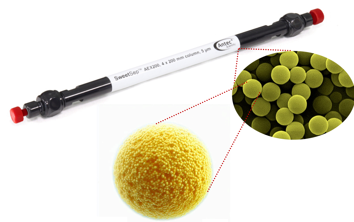
Figure 1. SweetSep™ AEX200 column based on a polymeric stationary phase consisting of monodisperse 5 µm particles coated with latex nano beads, functionalized with quaternary amine groups.
